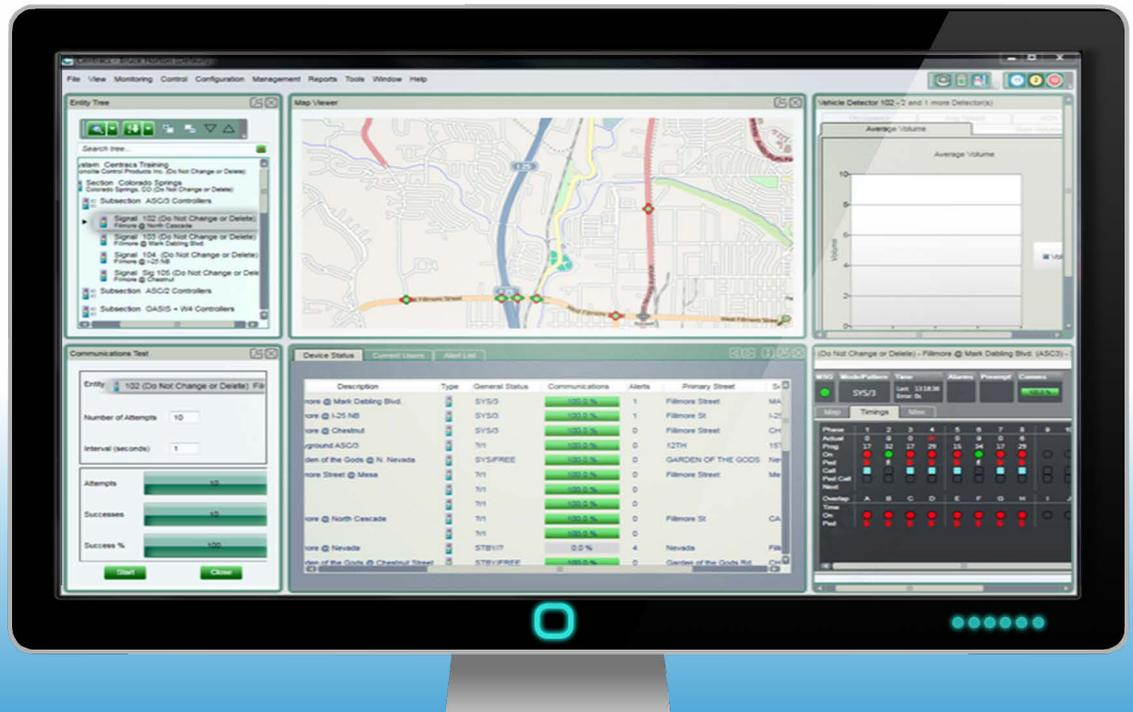
▶▶ Centracs MOE module provides these new tools for measuring and assessing factors impacting traffic signal coordination, as well as to satisfy performance measures evaluations.
