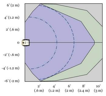
Adjustable radar detection zone. The purple area depicts the sensor detection zone for all vehicles (including bicycles). The green area depicts the sensor detection zone for large vehicles. The 4' (1.2 m) and 6' (2 m) arcs represent detection distance settings.
