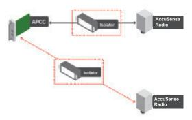
The minimum AccuSense Control system consists of an AccuSense Control, one AccuSense Radio, and a isolator. The system can also consist of two AccuSense Radios with an isolator for each AccuSense Radio that offers electrical isolation up to 1500V, surge protection up to 1500V, and AC power cross protection.
